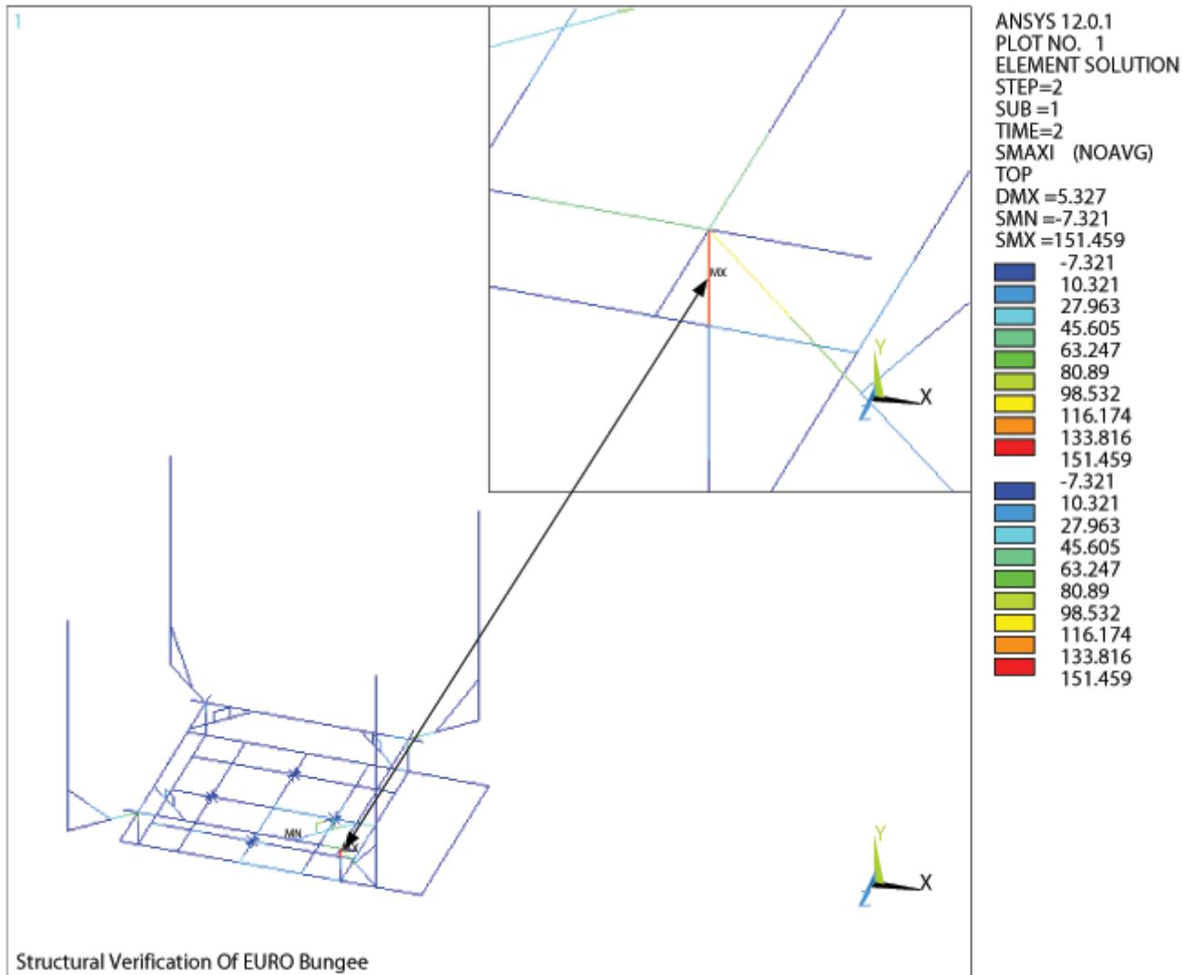
Figure 3.5 – Stresses In Steel Beam Structure, Due To Load Case 2
