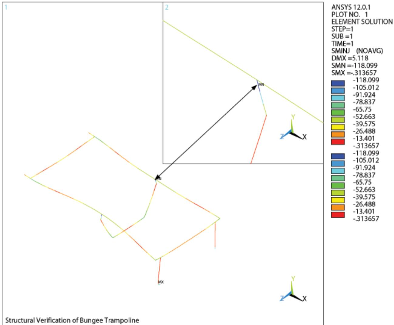
Figure 3.17 – Stress In Steel Beam Structure, Due To Load Case 1
