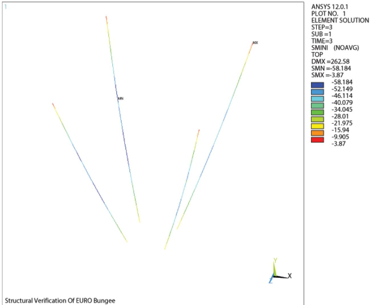
Figure 3.10 – Stresses In Aluminium Beam Structure, Due To Load Case 3
