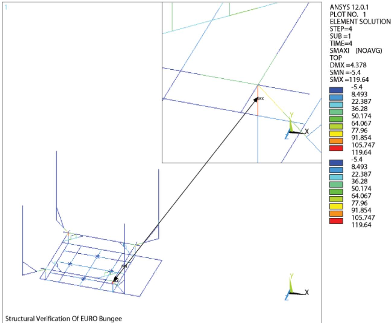
Figure 3.13 – Stresses In Steel beam Structure, Due To Load Case 4
