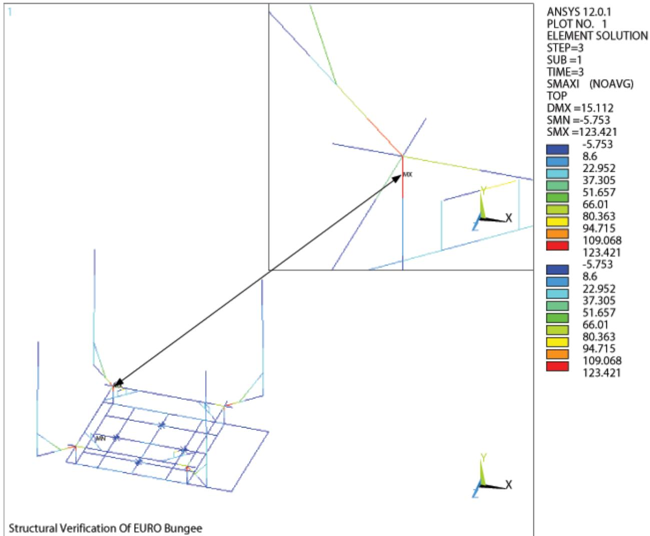
Figure 3.9 – Stresses In Steel Beam Structure, Due To Load Case 3
