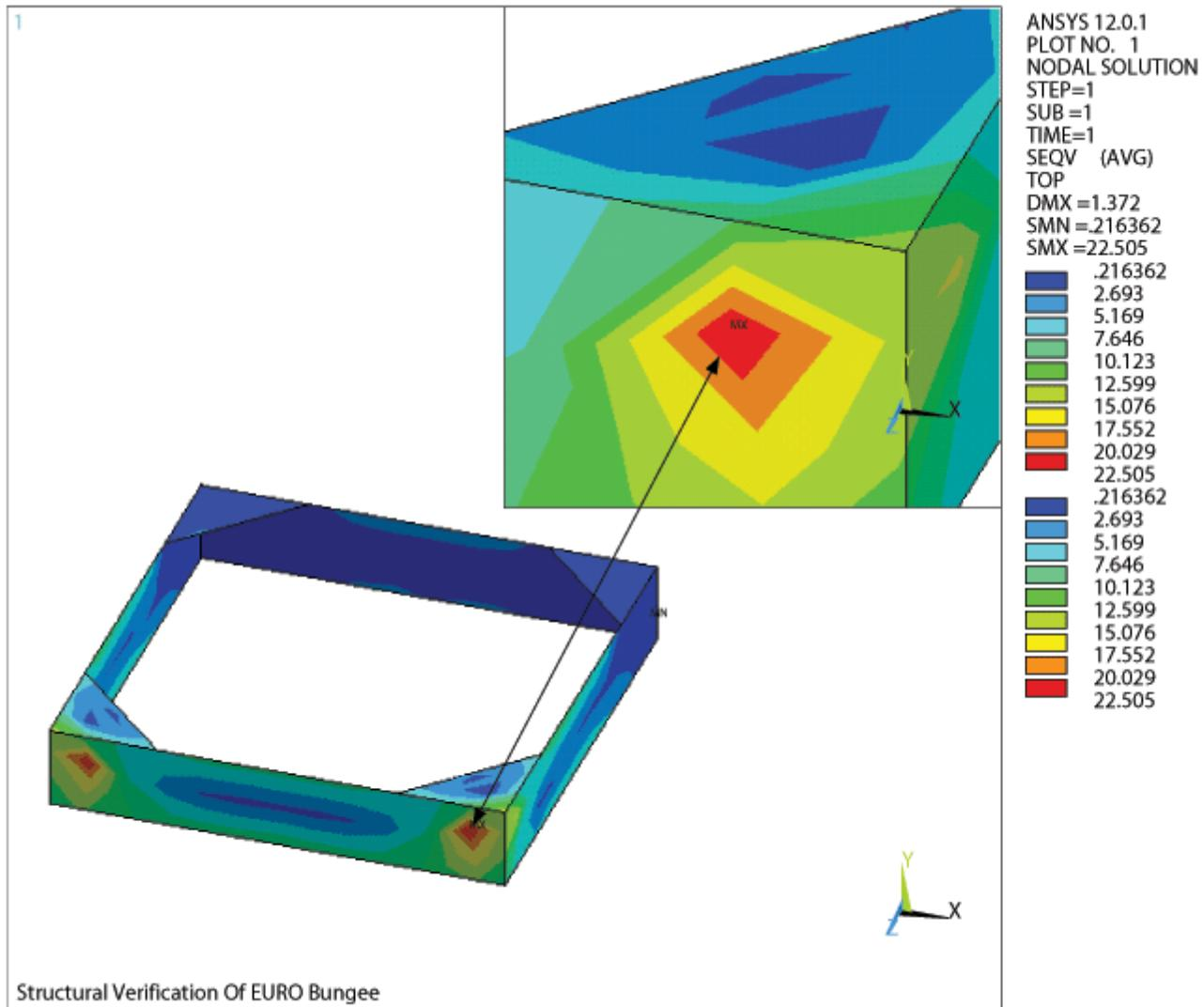
Figure 3.3 – Stresses In Steel Plate Structure, Due To Load Case 1
