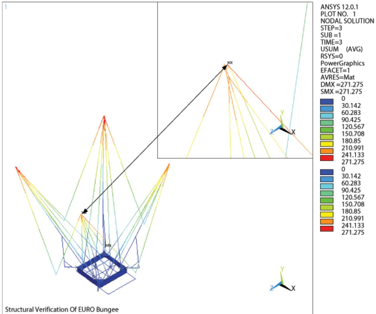
Figure 3.12 – Overall Deflexion In Structure, Due To Load Case 3
