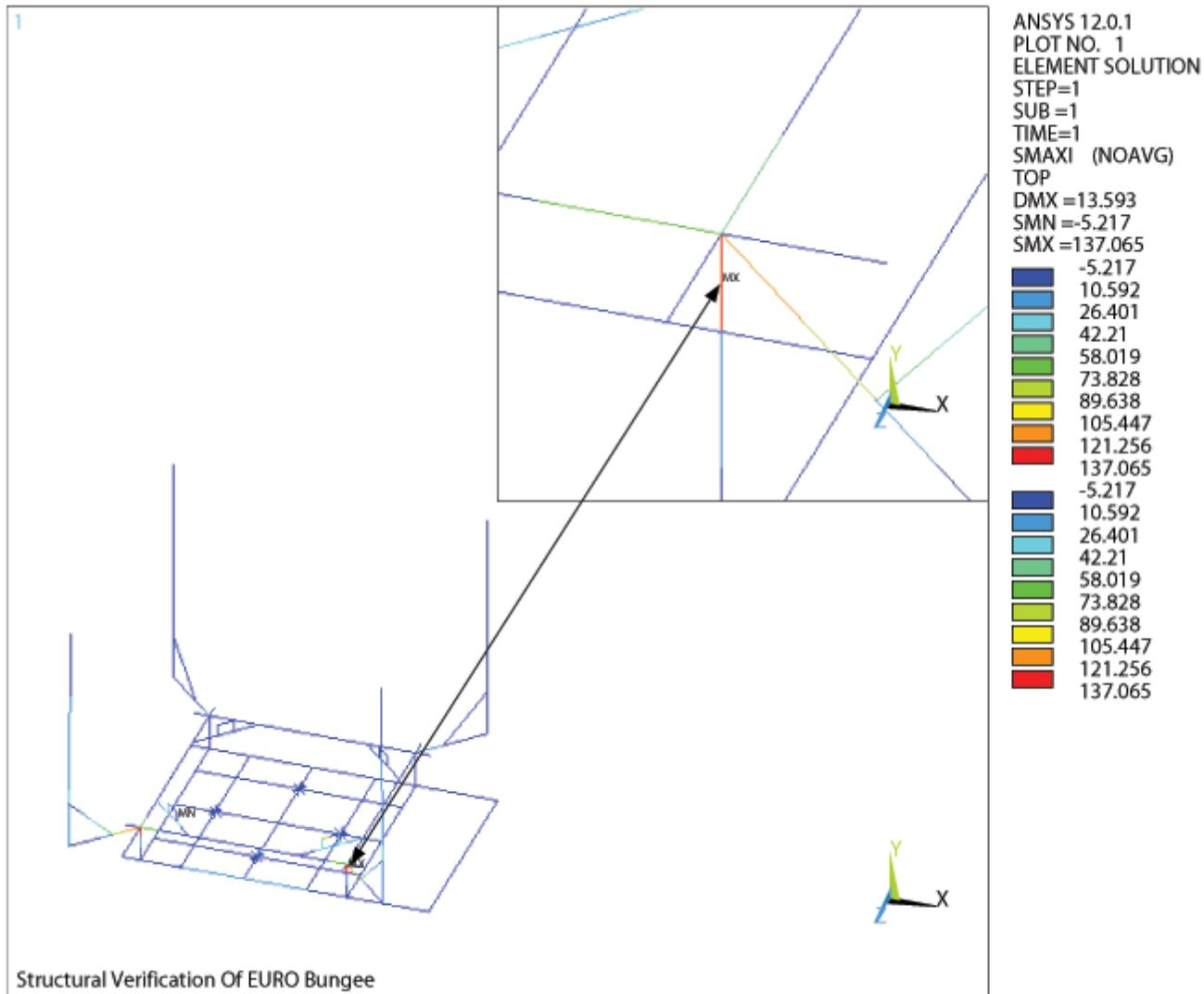
Figure 3.1 – Stresses In Steel Beam Structure, Due To Load Case 1
