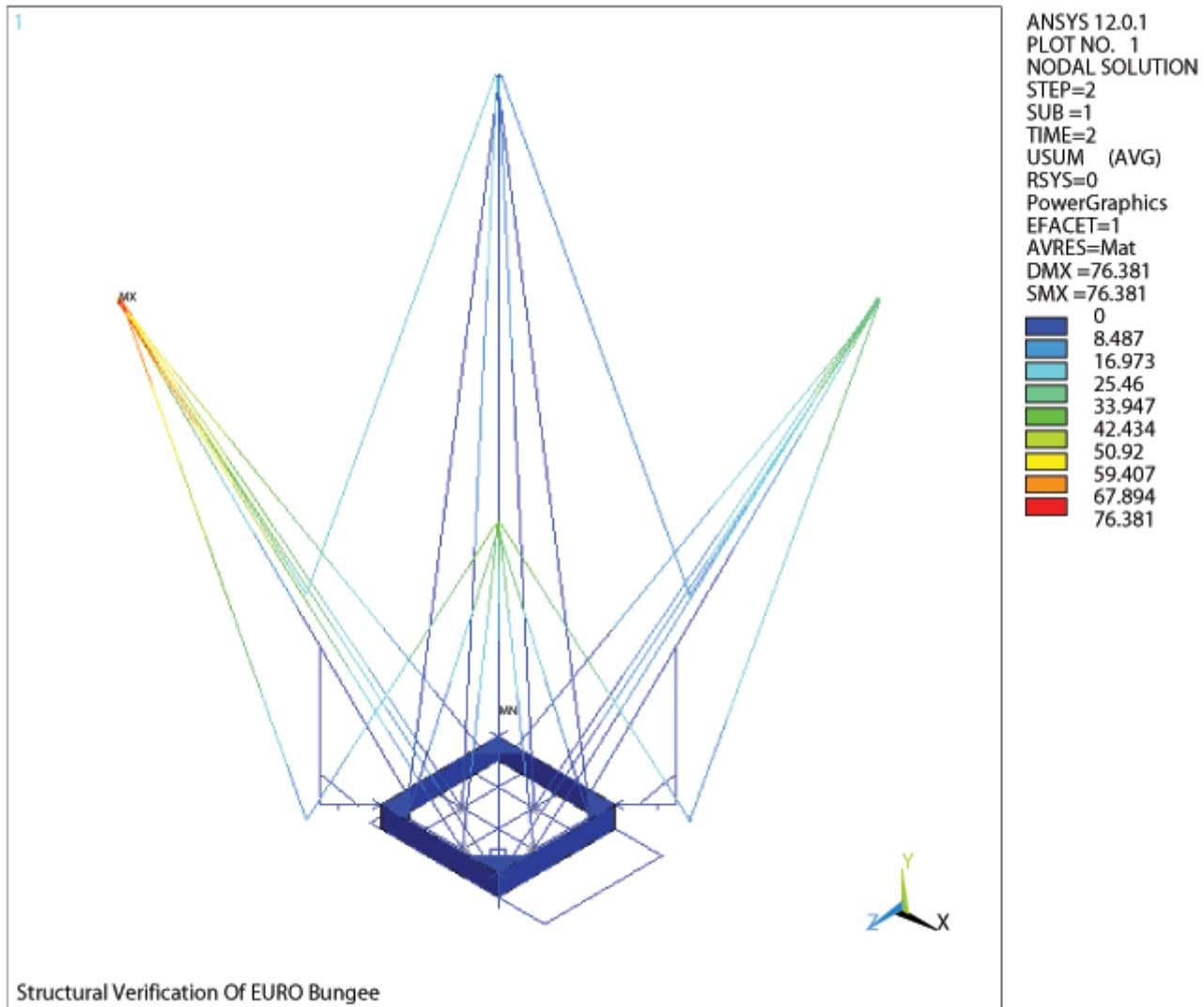
Figure 3.8 – Overall Deflexion In Structure, Due To Load Case 2
