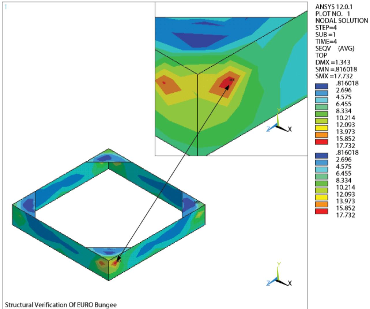
Figure 3.15 – Stresses In Steel Plate Structure, Due To Load Case 4
