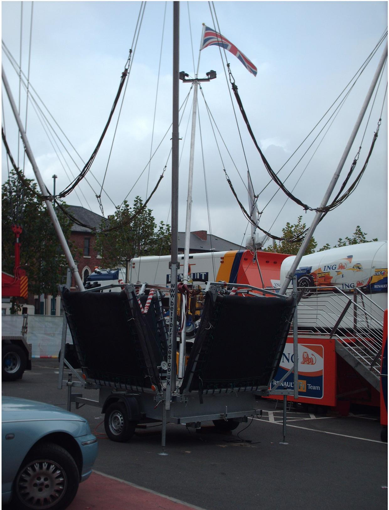
Figure 1.1 – Typical View Of 4-Person, Bungee Trampoline Device
