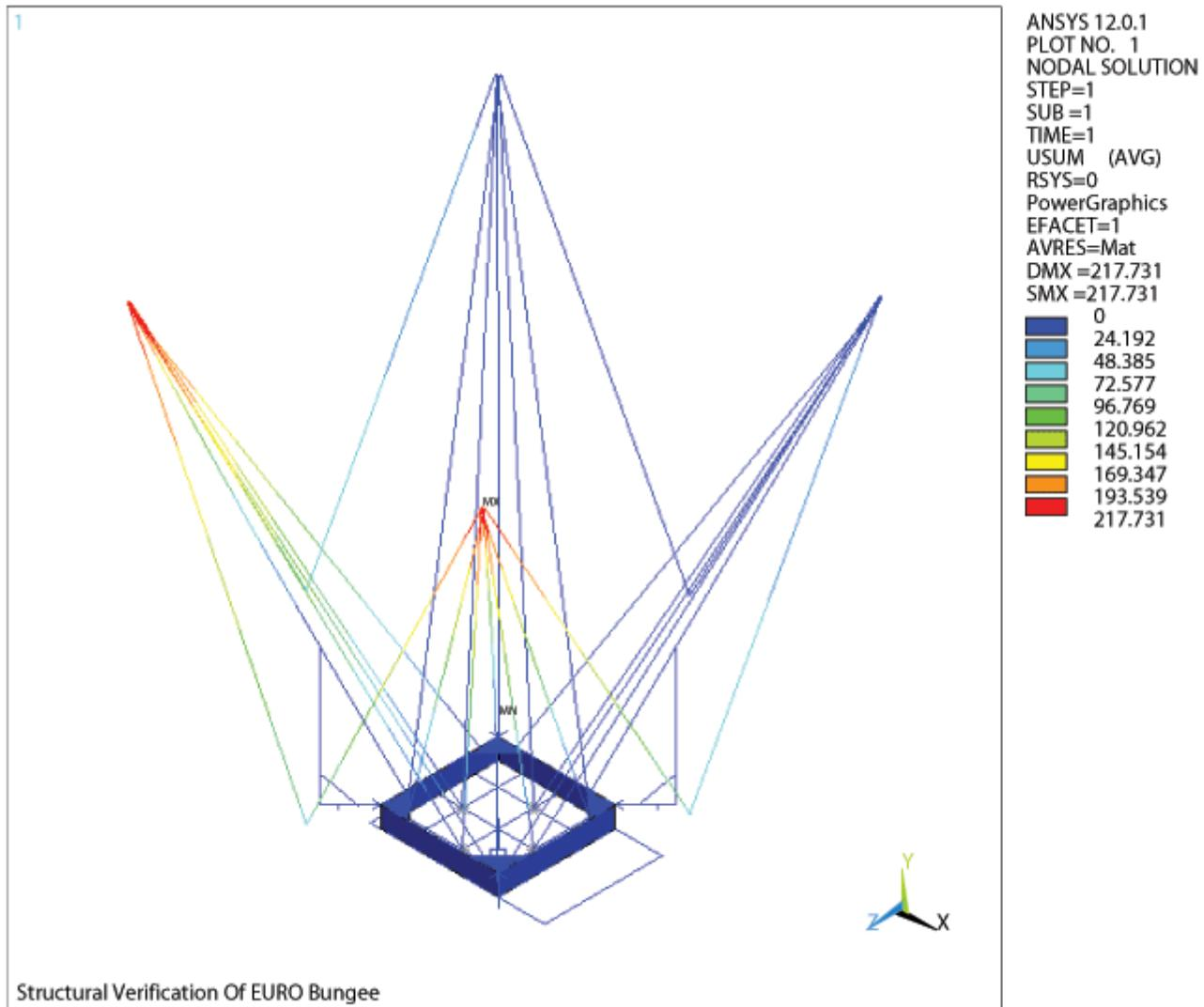
Figure 3.4 – Overall Deflexion In Structure, Due To Load Case 1
