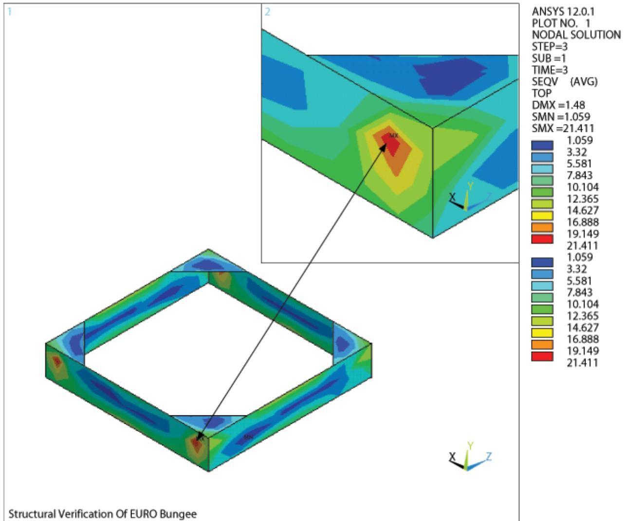
Figure 3.11 – Stresses In Steel Plate Structure, Due To Load Case 3
