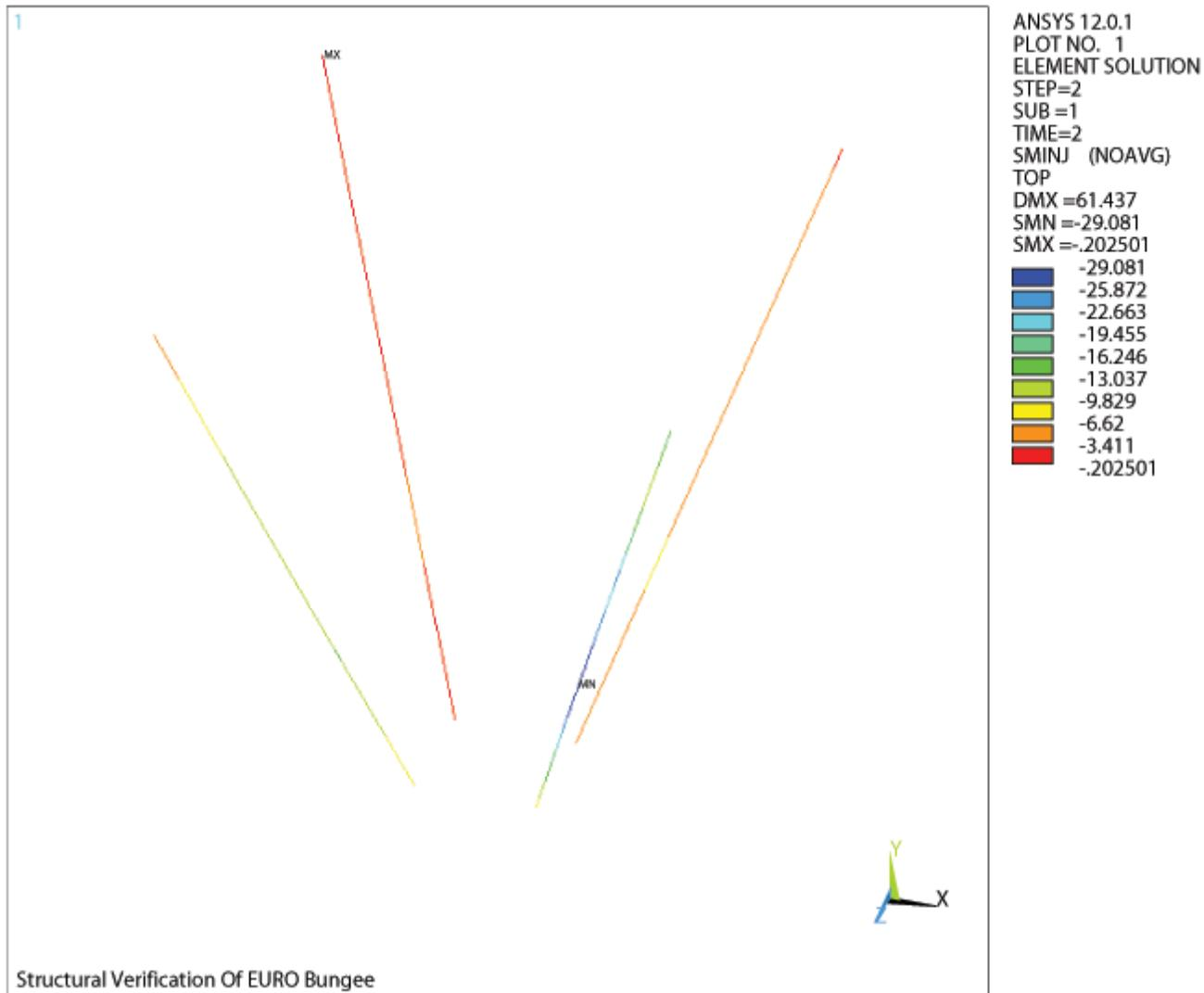
Figure 3.6 – Stresses In Aluminium Beam Structure, Due To Load Case 2
