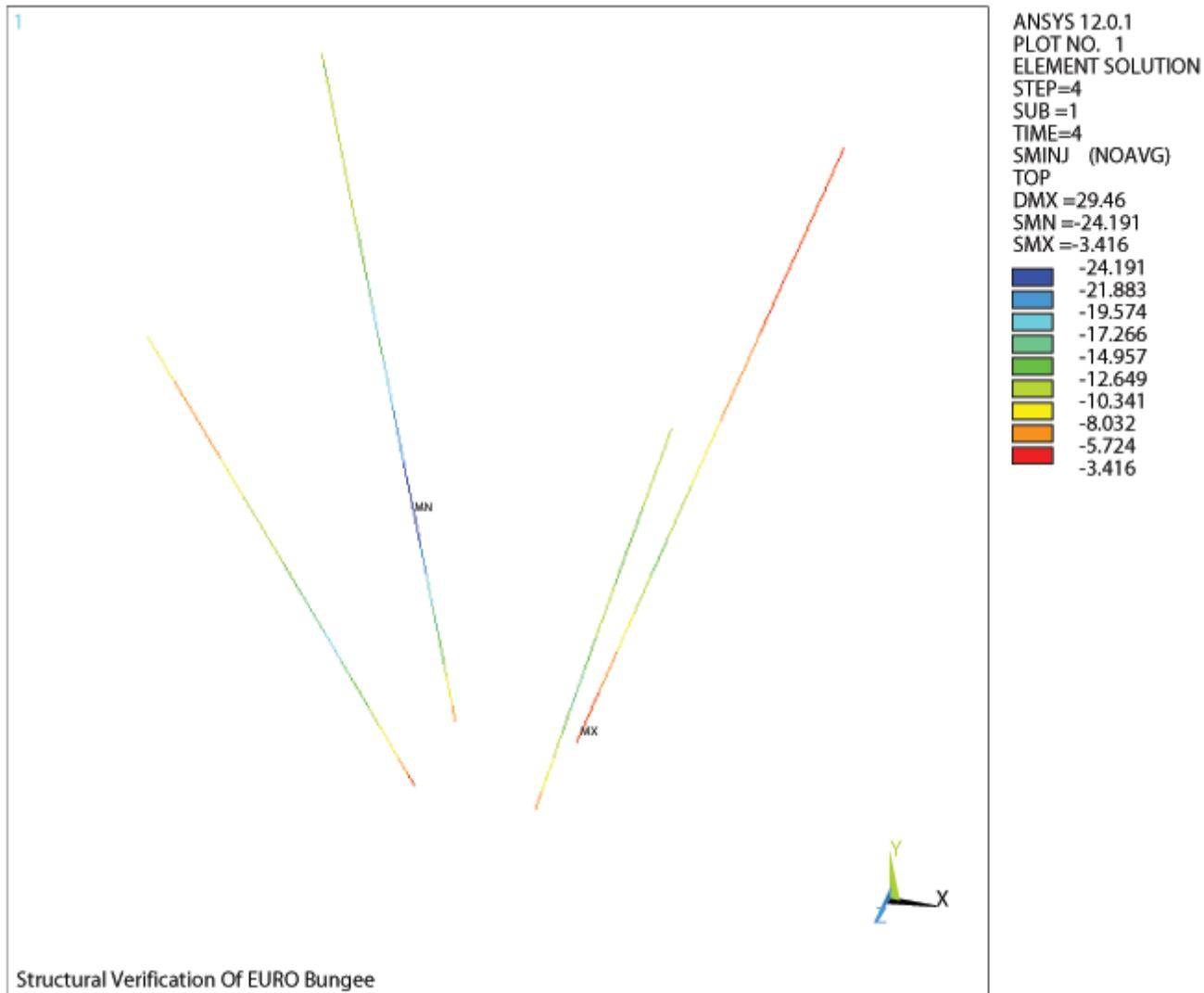
Figure 3.14 – Stresses In Aluminium Beam Structure, Due To Load Case 4
