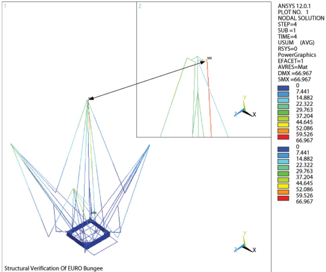
Figure 3.16 – Overall Deflexion In Structure, Due To Load Case 4
