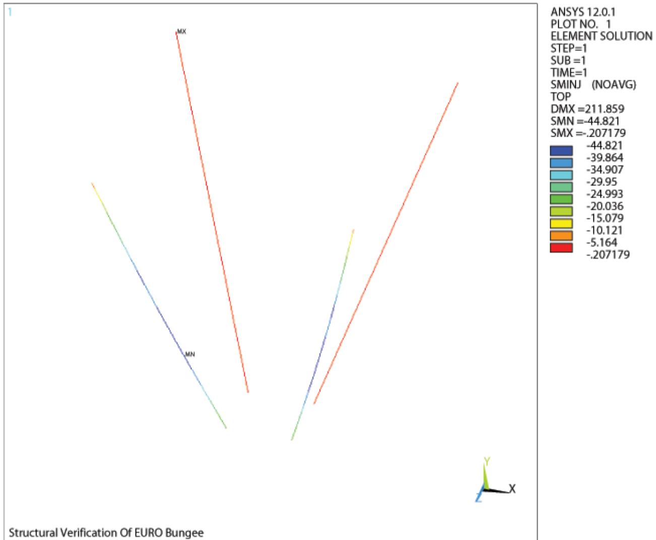
Figure 3.2 – Stresses In Aluminium Beam Structure, Due To Load Case 1
