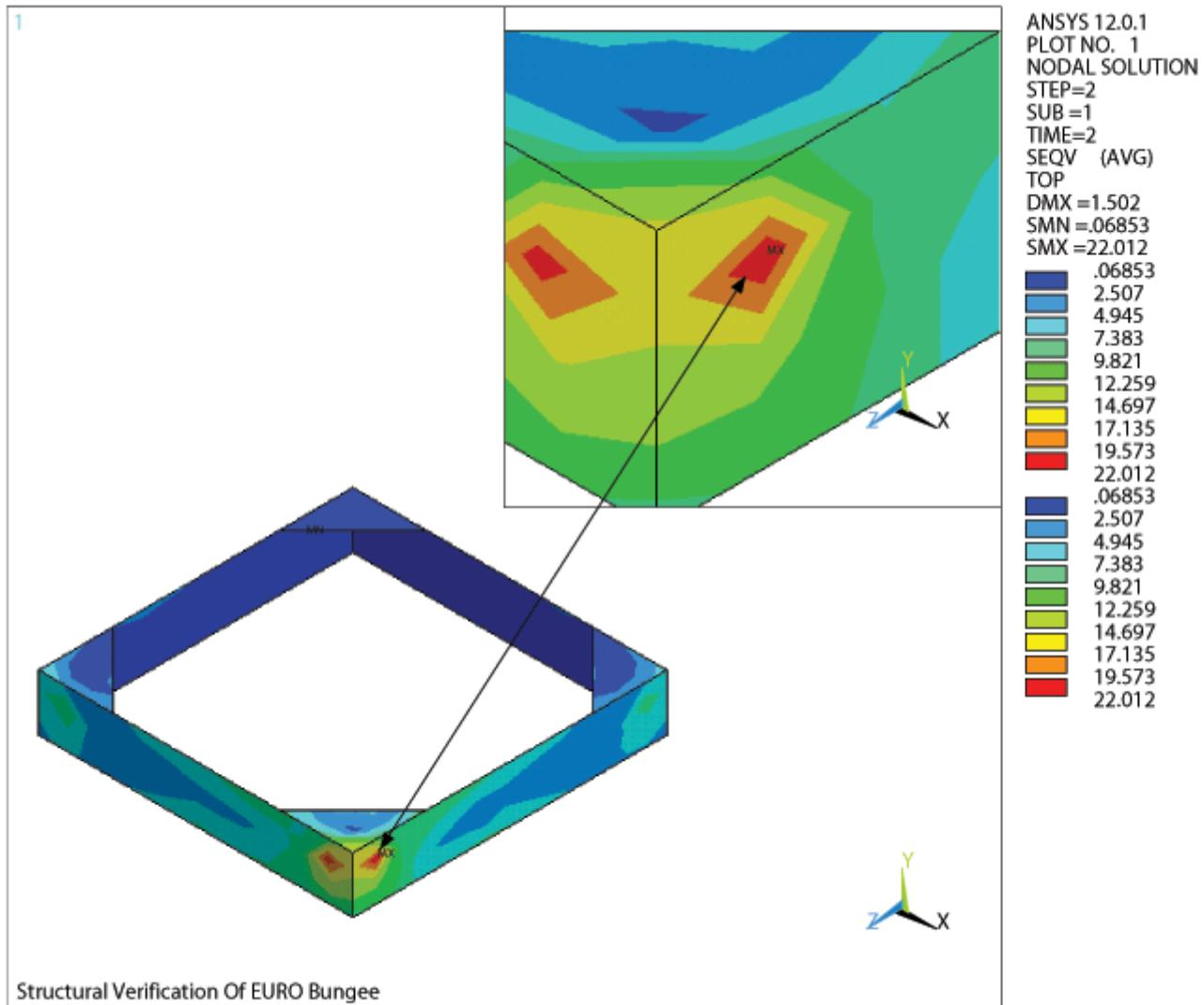
Figure 3.7 – Stresses In Steel Beam Structure, Due To Load Case 2
