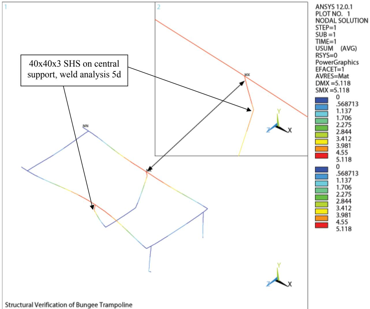
Figure 3.18 – Overall Deflexion In Structure, Due To Load Case 1
