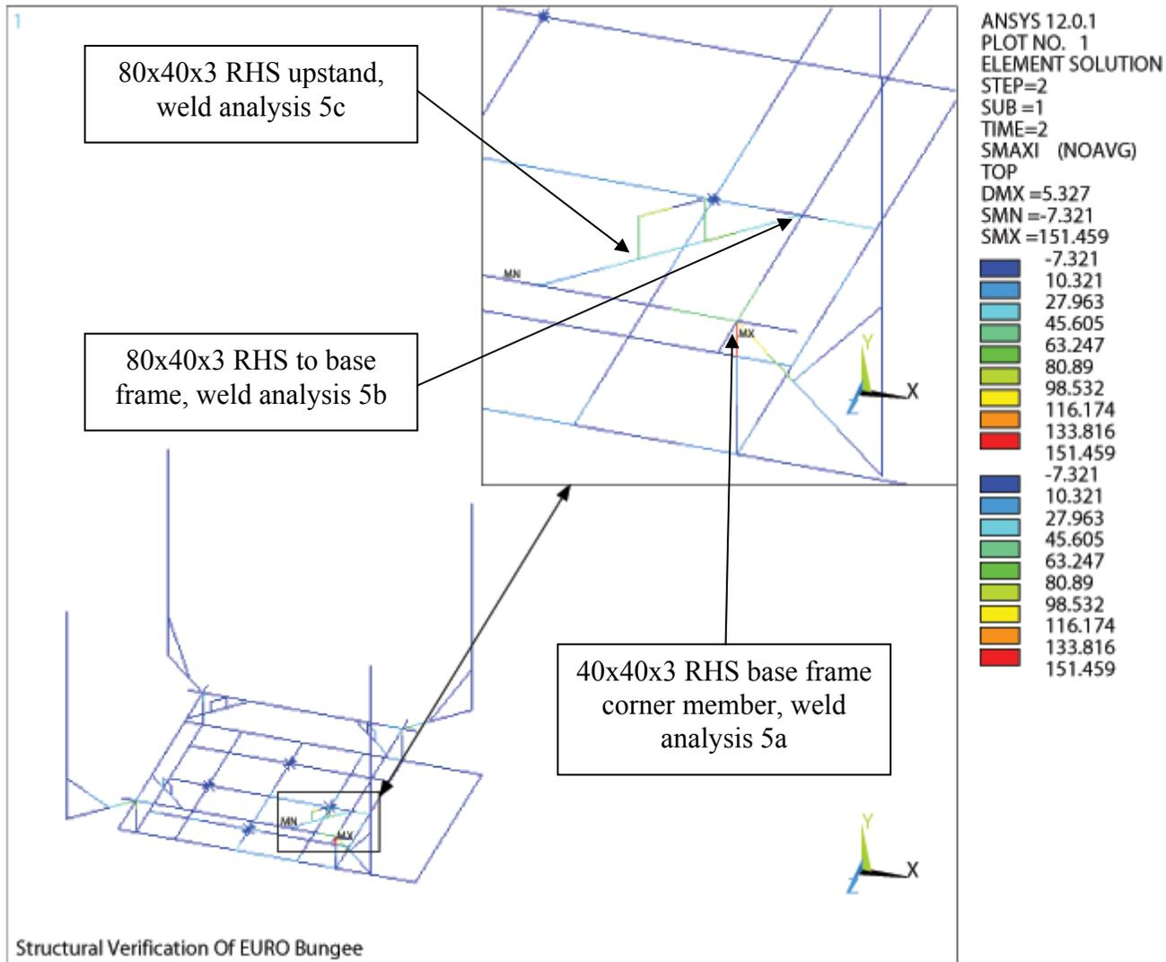
Figure 4.1 – Critical Welds
