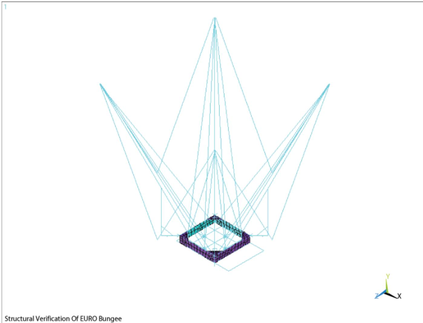
Figure 2.1 – Finite Element Model Of 4-Person Bungee Trampoline
